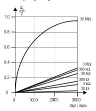
Voltage U., at measured resistance Rx relative to measuring range and display
