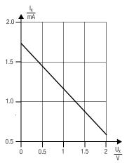
Measuring current L relative to displayed voltage value U. for the device under test
